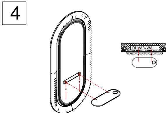
The table is placed in the slot of the glass holders and fixed with 2 adjustment fixing screws.
