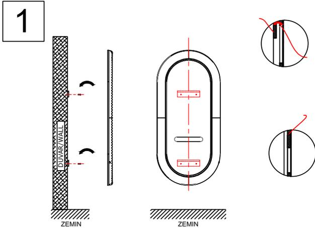
2 hanging brackets are fastened to the wall with 4 6x80 screws. Before the mirror body 45 is attached to the hanging apparatus, the LED sortie is pulled from the socket gap and the mirror is hung.
