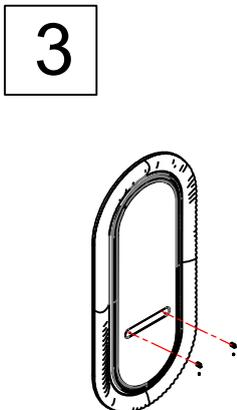
Center 2 glass holders in the middle area of the mirror and tighten them equally with 4x40 chipboard screws.
